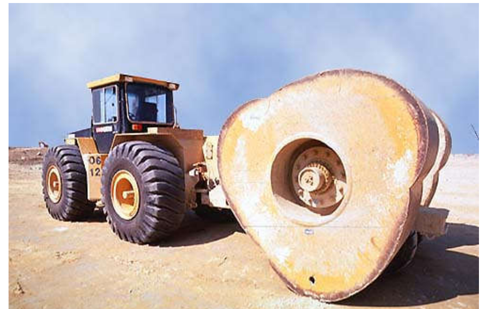
Impact Roller to Compact the Ground
