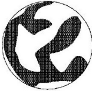
Fig. Schematic of structures observed in the early stage of phase separation in a polymer blend by (a) spinodal decomposition and (b) nucleation and growth
